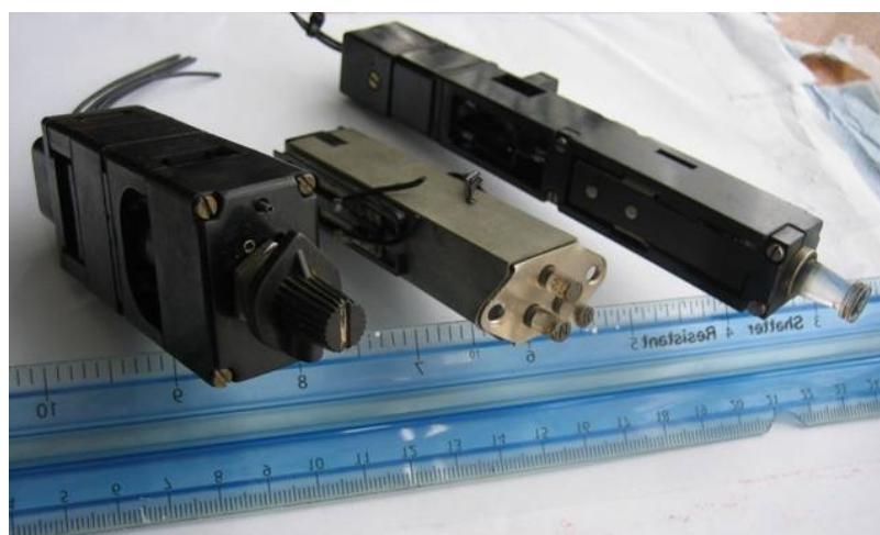
Figure 135 - Westinghouse miniature components, left to right: IPS thumb switch, IPS point indication light funnel unit, NX push-button. © Andrew K Overton
