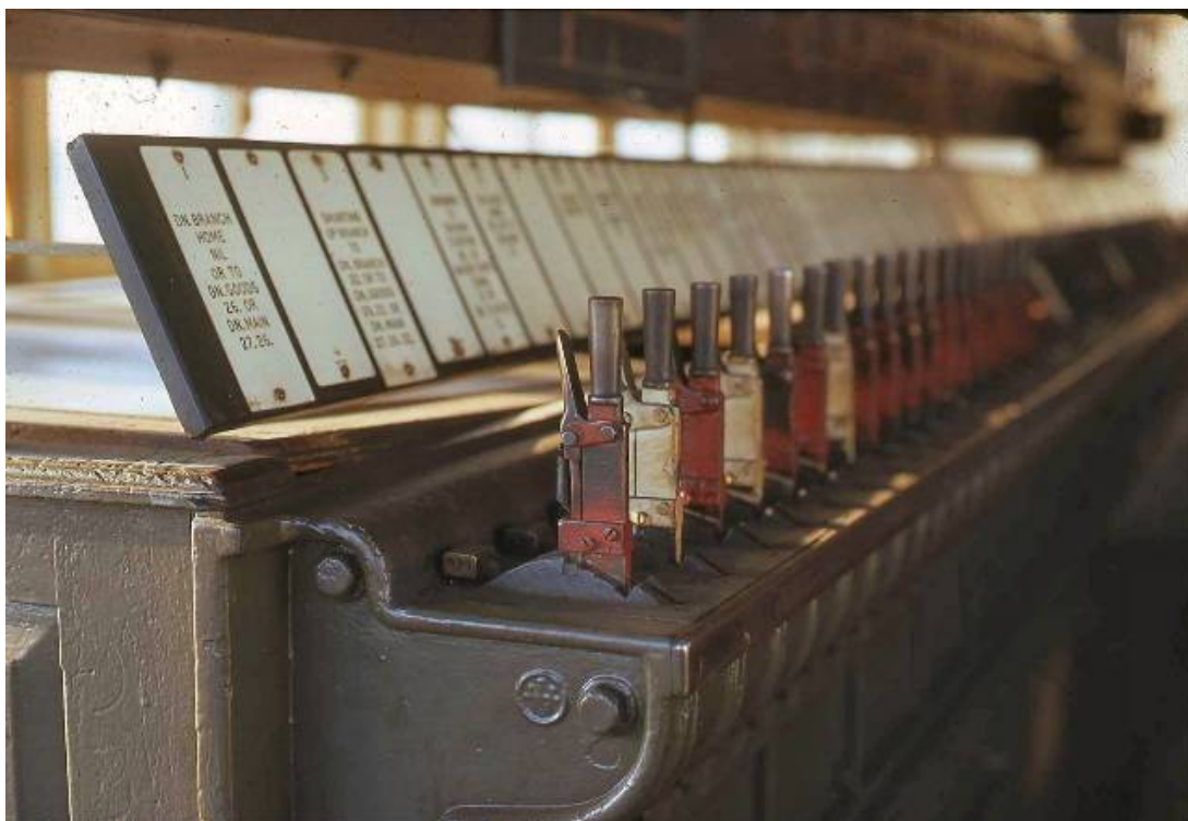
Figure 168 - McKH&W Style A PF(L), Green Lane. © John Boyes Collection
