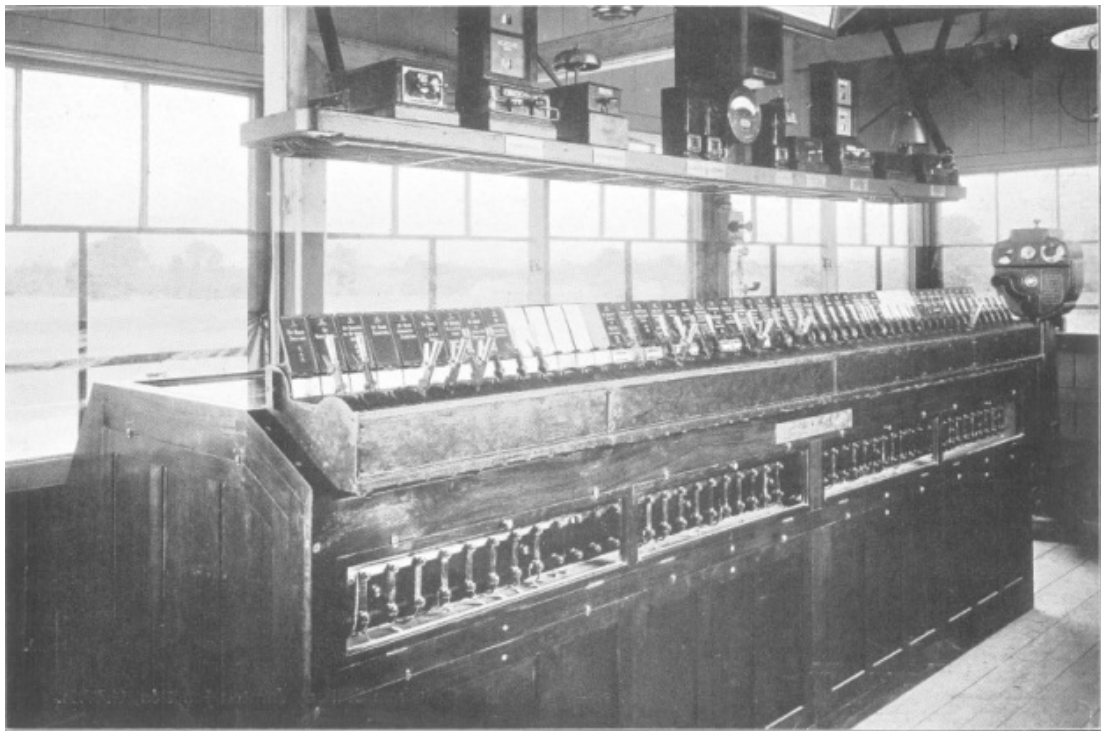
Figure 181 - Westinghouse M1 PF(L), Yarnton Jcn. © Siemens.
