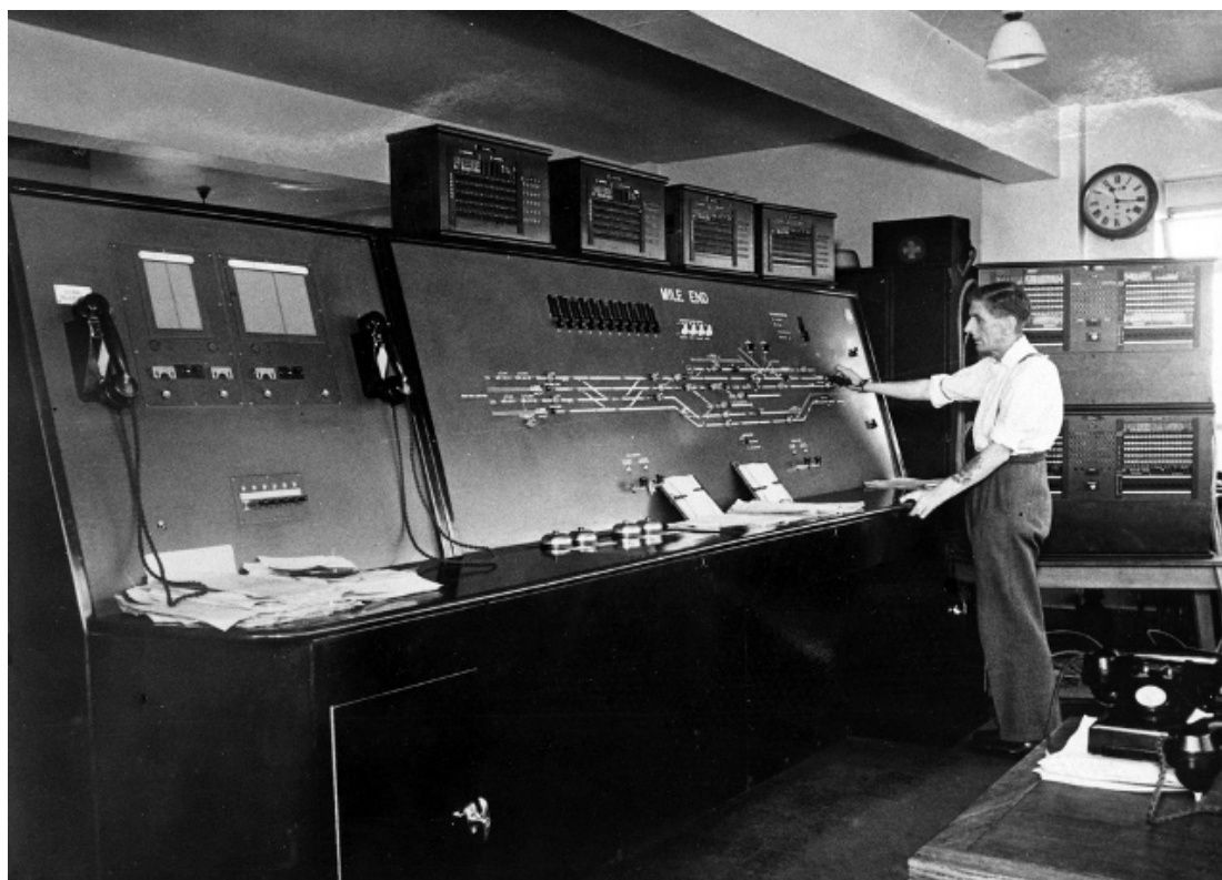
Figure 84 - MV-GRS NX(TP)[+], Mile End. © Beechwood Photography
