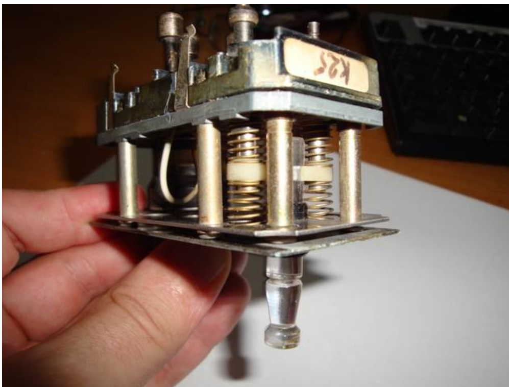
Figure 149 - Westinghouse M3 NX(PP)[+] tile top unit showing push-button assembly. © Brian Hornsey
